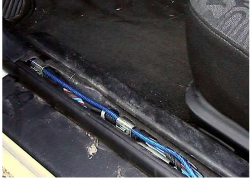
5) After lifting this up, run the wire under it, you should get something like this. Run this wire, in any way possible, all the way to the trunk of your car.
