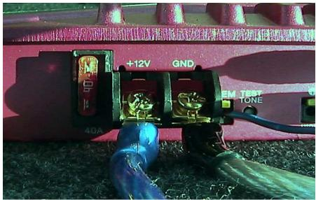
14) Now clamp the ends on the end of the wire and attach it to the amp, like so.
