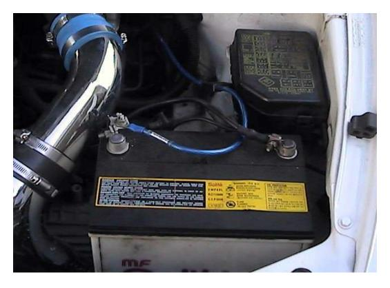
First thing to do is to do disconnect the battery. Then take out the fuse from your power wire. Next, put the power wire close to the battery, but do not connect it yet.
