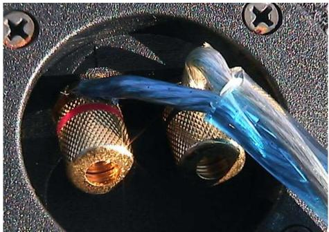
14) Ok, on the back outside of the box, you'll find these, attach one end of a new wire to this.
